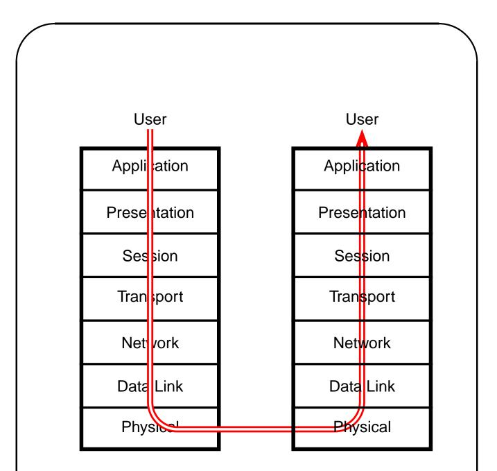
When the message reaches the receiver's hardware, it starts moving **up** until it is handed to the receiving application.
